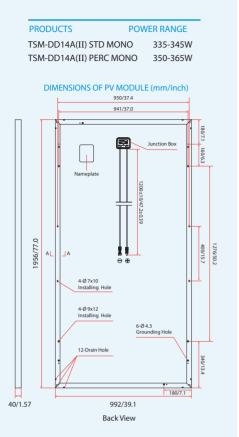
11/0.43 Silicon Sealant Laminate Frame 35/1.38 (A-A)
